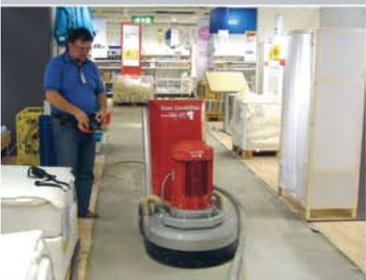
Scan Combiflex 700 RC sköts enkelt via radiostyrning.
