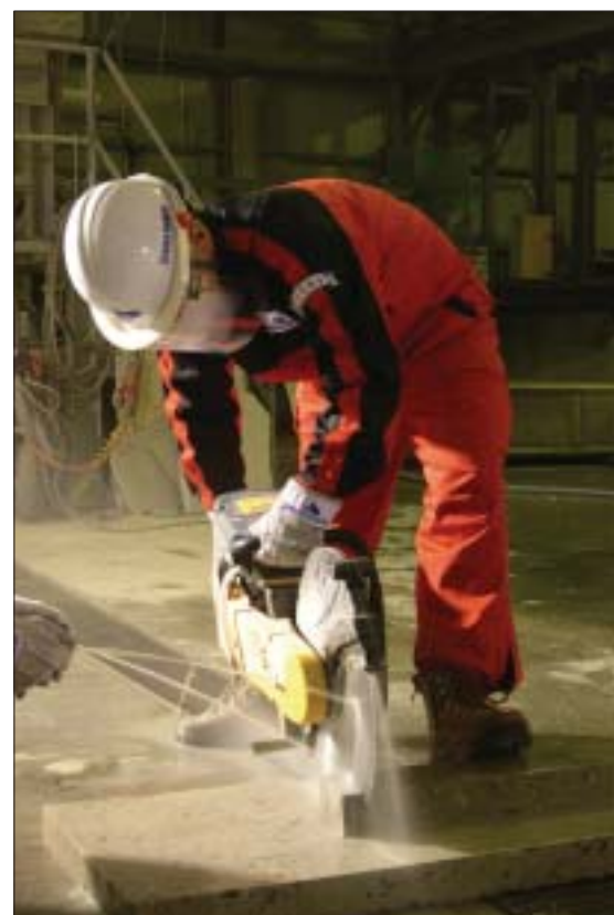
Fig 5 Tests showed that cutting with an ARIX segmented blade was faster and more efficient than conventional segmented blades
