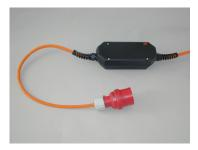
The DK 42 A is switched by an on-off button on the top of the machine via a conductor. For saving weight it is fitted in a cable case. By this device the motor is solidly and exactly switched and the required undervoltage trip is realized.
