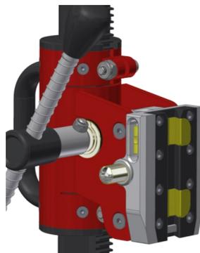
40<sup>+</sup> drill carriage with universal motor mounting is both strong and compact.
